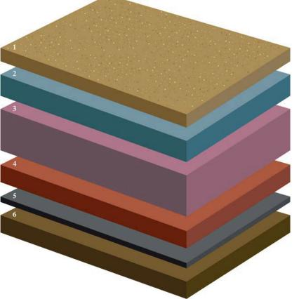
I. Clearmac® cold-applied paving surface: I 6mm layer depth for 3mm size aggregate, I 8mm layer depth for 6mm size aggregate, 24mm layer depth for I 0mm size aggregate.
