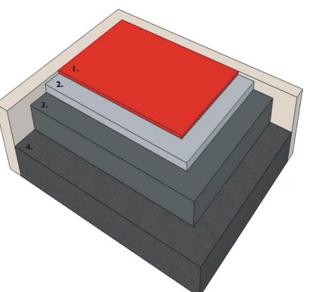
**I. Playsafe® top:** I 5-20mm surface layer of coloured EPDM rubber crumb.
