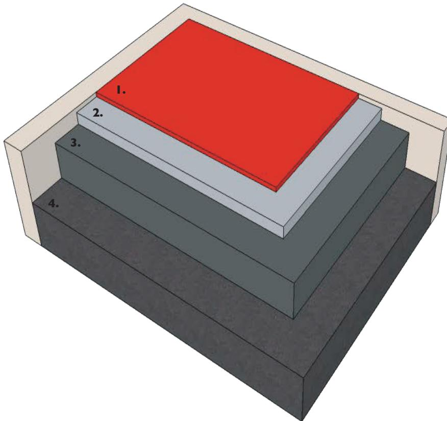
**1. Playsafe® top:** 15-20mm surface layer of coloured EPDM rubber crumb.
