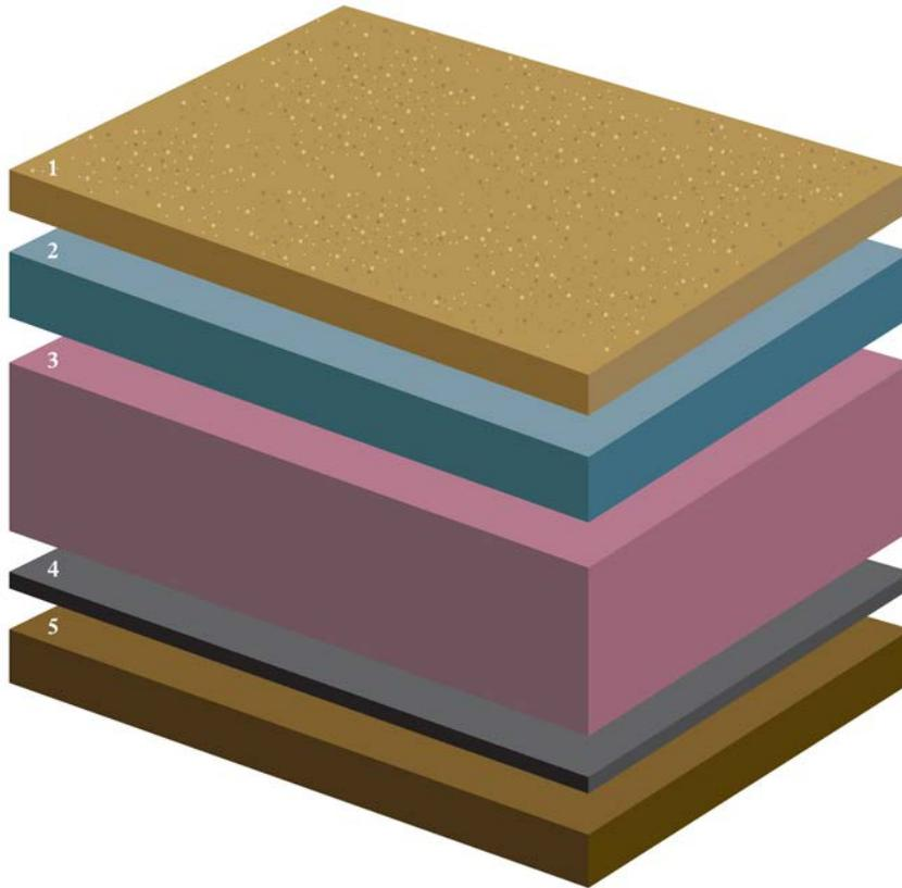
**1. Clearmac® cold-applied paving surface:** 12mm layer depth for 3mm size aggregate, 16mm layer depth for 6mm size aggregate, 22mm layer depth for 10mm size aggregate.
